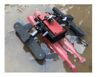
The new AmphiSTAR robot from Ben Gurion University swims, crawls over rough ground using a sprawling mechanism inspired by cockroaches, and runs over water like a basilisk lizard, the designers say.
