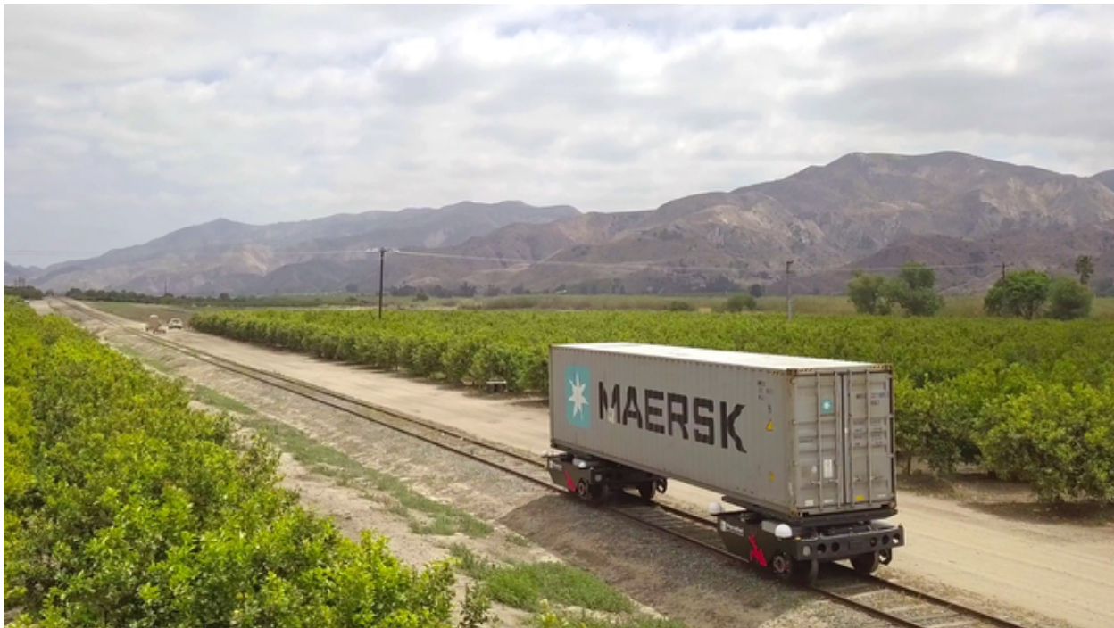
Parallel Systems' smart flatbed rail cars moving a cargo container.
